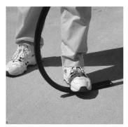
Pre-bend the first few feet of the track (by stepping on it and holding for 30 seconds) curved in the same direction as the rest of the coil.
