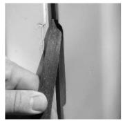
As necessary, file the edges of the mast gate opening until they are smooth-particularly the upper inside edges.
