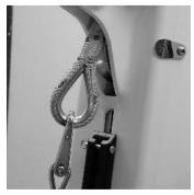
Pull the track down 1 to 2 inches from this point. Make certain the top of the track is clear of any masthead fittings.
