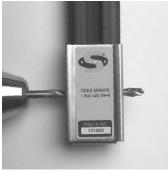
Place the stainless cover over the cut end of the track and clamp in place. Using the holes in each side of the cover as guides, drill a 1/4 " hole (bit provided) through the track.
