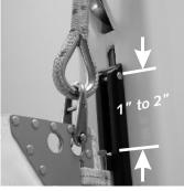
Raise mainsail and check that the headboard slide does not contact the quick pin at the top of the track. There should be 1" to 2" clearance. If necessary adjust the track position.
