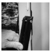
Slide the top of the track through the mast gate on centerline and guide upwards. Once the track is started, remove the other tie wraps in sequence as needed.
