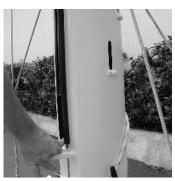
Press bottom of track against mast to determine cut off point (minimum of 3 inches above gooseneck).
